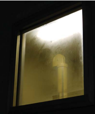
A lead glass surface discolored because its surfaces was leaved wet condition.
